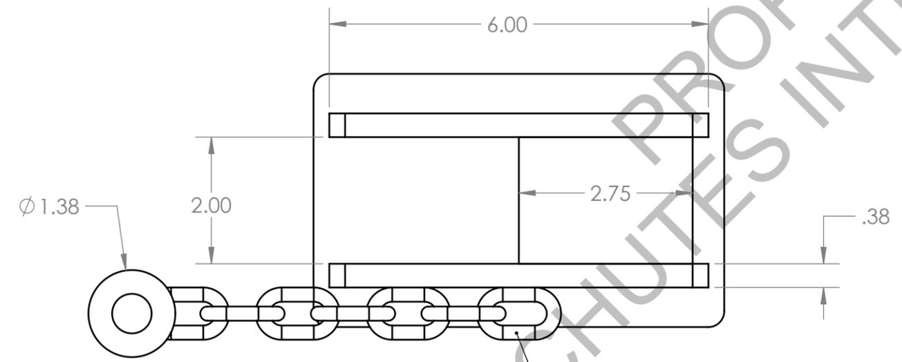
**NOTE** :CHAIN WILL BE WELDED ON OPPOSITE SIDE FOR LEFT SIDE DP600 CONNECTOR
